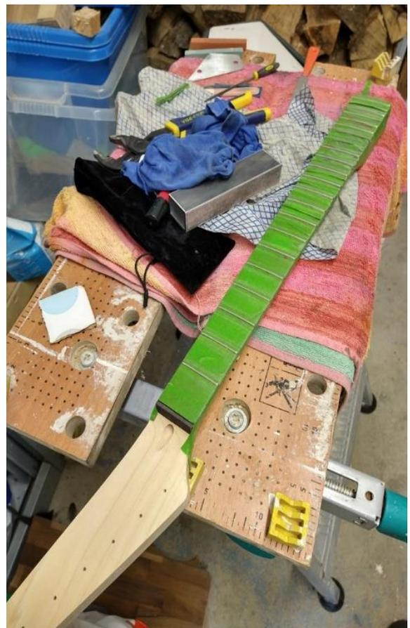
It's not really necessary but I used sanding sealant on the neck after sanding it all smooth, resanded and applied some trusty Osmo PolyX with the headstock decal applied between the first couple of coats. I bonded, levelled and polished the frets.
